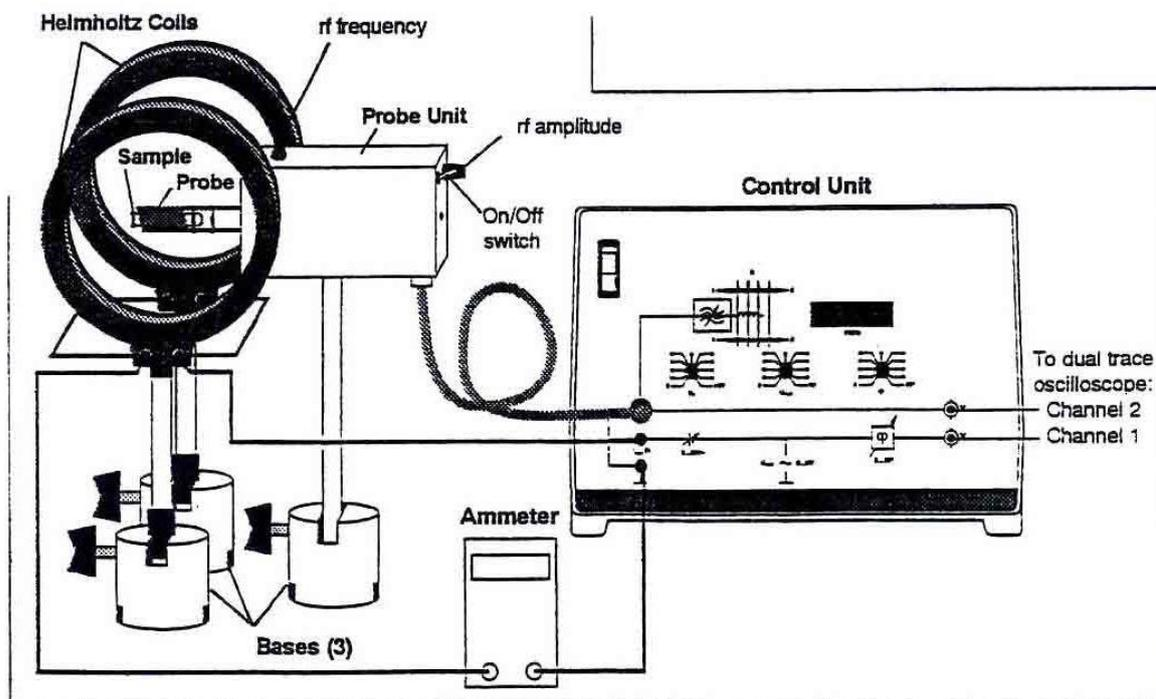
Figure 9 Setup using the Control Unit
